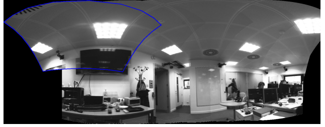
Figure 4. An example spherical panorama produced by tracking the camera rotation using CNN features
